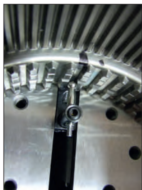
Carbide ball head for the control of teeth on a measurement table.
