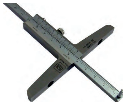
Additional cylindrical stop for the control of depth of a position in a bore.
