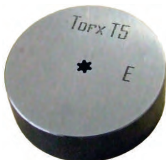
Master ring gauge for the control of Torx ® profile to customer specifications.
