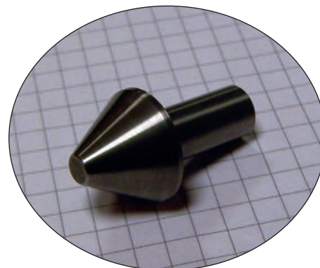
Conical carbide heads for the control of distance between centres on a measurement table.
